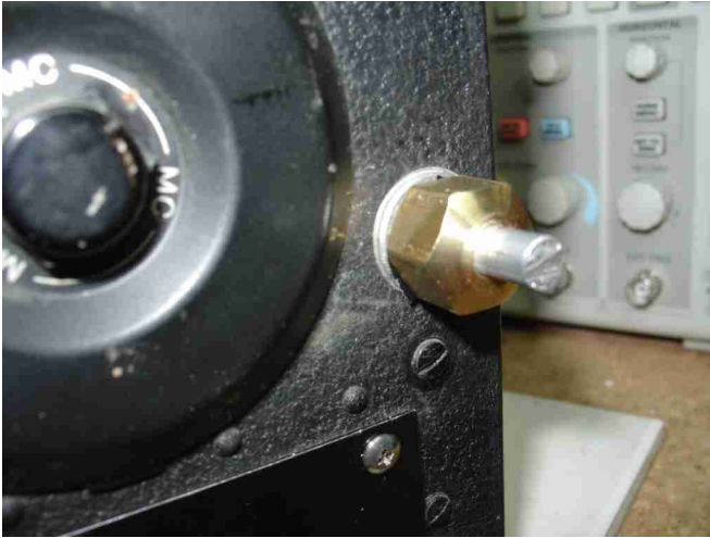
Photo G: Shaft adapter/extension in place
