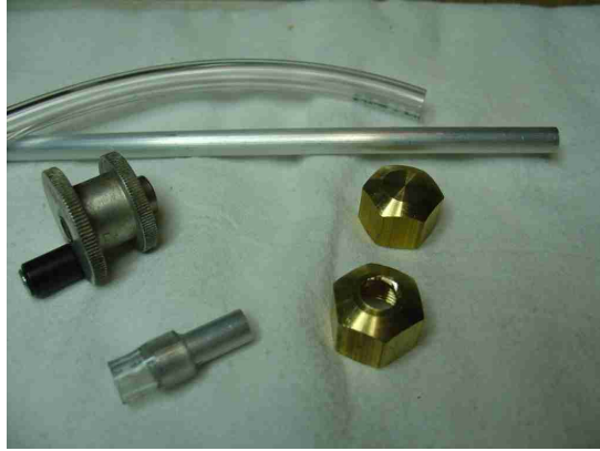
Photo F: Plastic tube, 1/4" rod, 3/8NPT cap, and final shaft adapter/extension (lower left)
