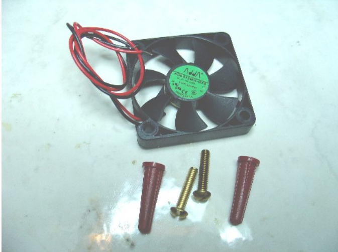
Fan (50mm) and Anchors
