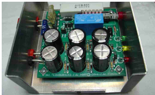
Photo F: Six 25-farad capacitors in series!
