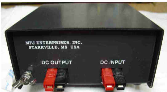
Photo G: Added ground post
