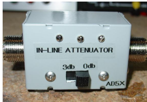
Photo H: 3dB attenuator outside view
