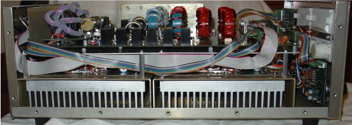
Photo C: Individual 600-watt amplifier heatsinks. Left-side view.
