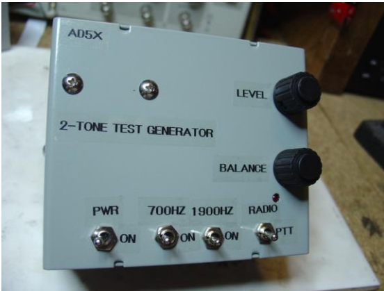
Photo G: 2T-gen external controls
