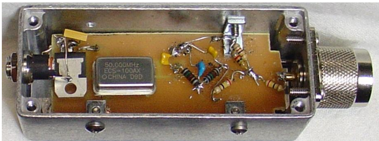
Photo B: Internal view of the 50 MHz reference oscillator. Pretty simple!
