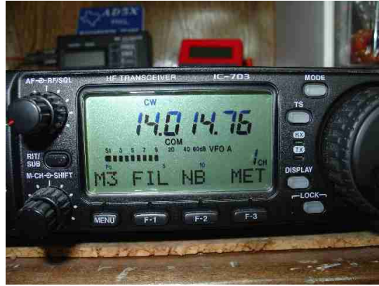
IC-703 S-meter reading with 82 dB in-line
