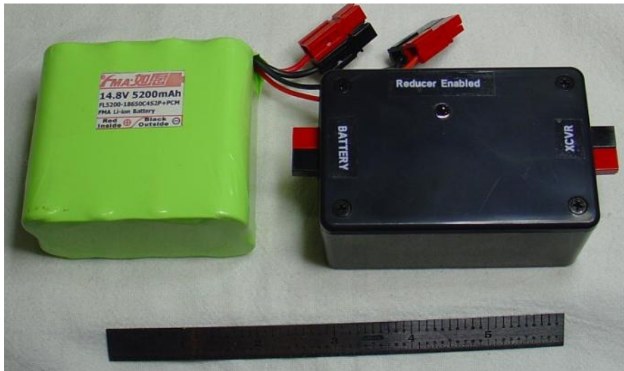
Figure 5: Assembled voltage reducer & Sanyo 5200mah LiPo battery
