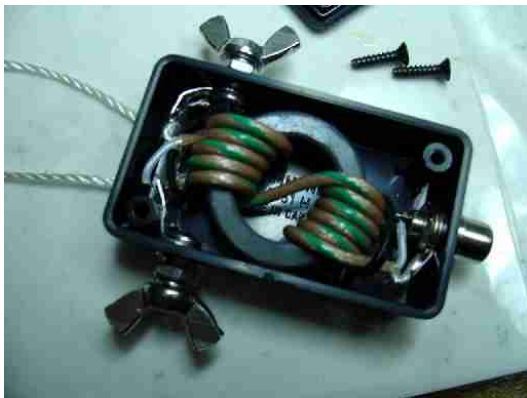
Photo A: Balun In Box
