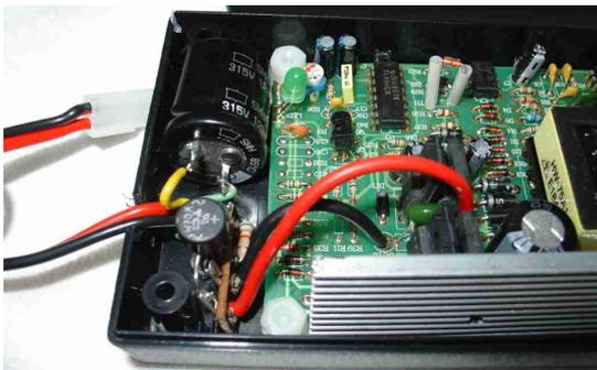
Photo C: Close-up of rectifier circuitry
