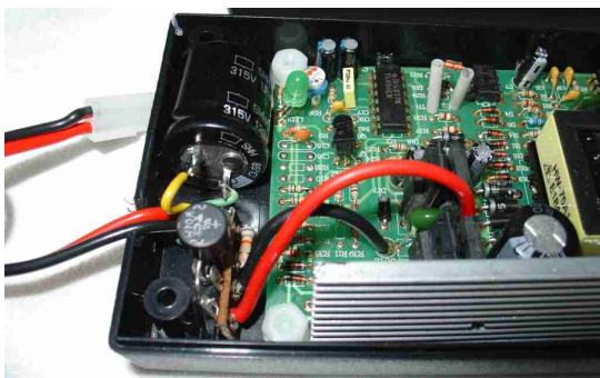
Photo C: Close-up of rectifier circuitry
