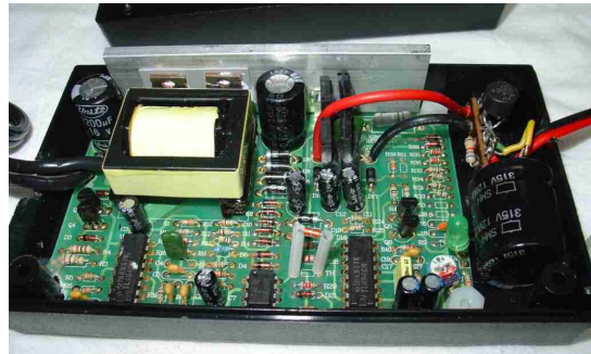
Photo B: Remounted 12V/120VAC inverter
