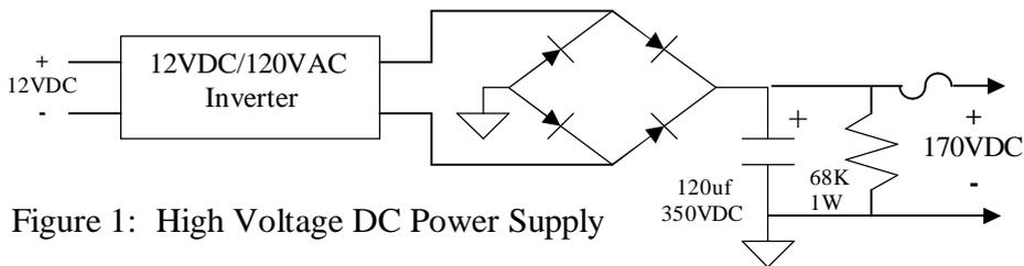
Figure 1: High Voltage DC Power Supply
