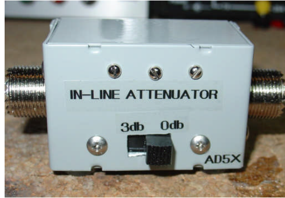
Photo H: 3dB attenuator outside view
