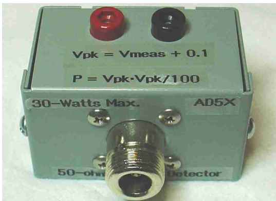
Photo C: Completed 30-watt detector/load
