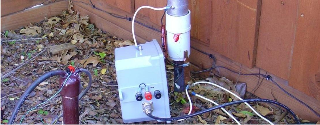
Photo D: Matching unit at the base of the author's 43-foot antenna (strapped for 80 m)
