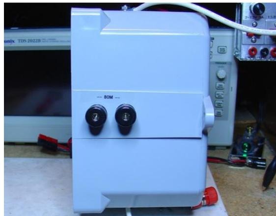
Photo C: 80 Meter Coil Shorting Posts
