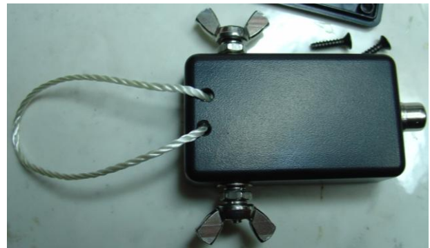
Figure 4: Nylon support string
