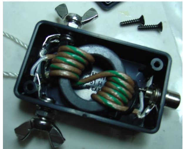
Figure 2: Balun mounted in plastic box
