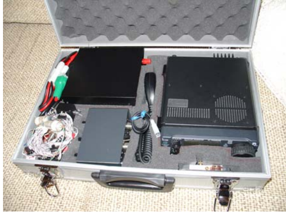
The complete portable station in the MFJ-6404
