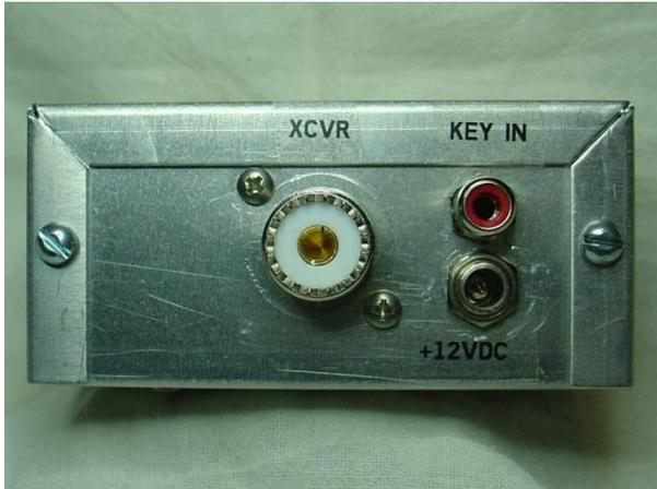
Figure 5: Transceiver side
