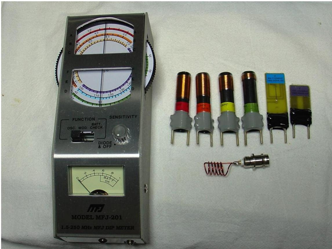
Photo D: The MFJ-201 Grid-Dip Oscillator
