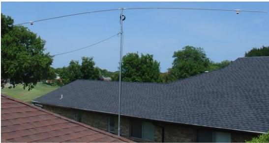
Photo E: Completed 17/12M trap dipole
