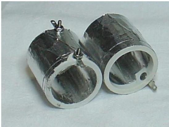
Photo A: Home-built Trap Capacitors
