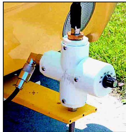
Figure 8—The completed assembly, consisting of mount, bracket, feed line and antenna, attached to the car and "ready to roll."
