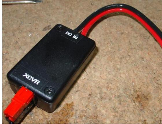
Photo D: Final cartridge fuse assembly
