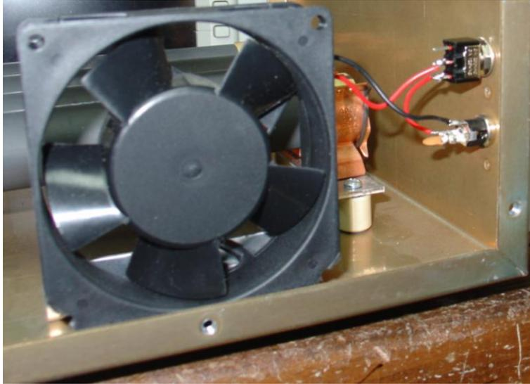
Photo B: Fan On/Off switch Internal View
