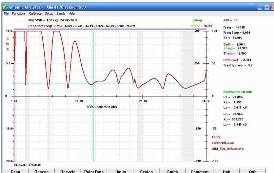
**Photo D:** 1.7-29 MHz SWR swept response of the Butternut vertical.
