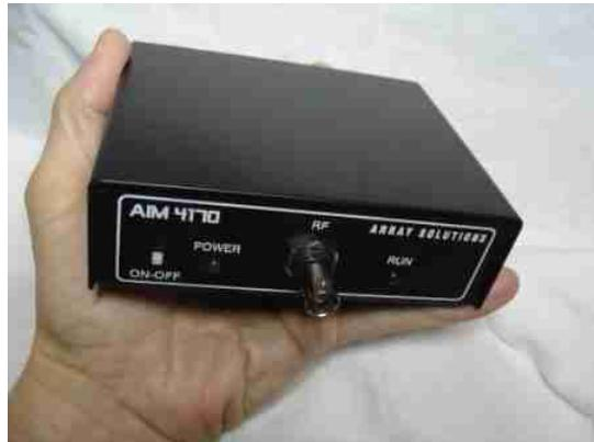
**Photo A:** The compact AIM 4170 does and everything and more than you'd expect from a full-featured antenna analyzer.
