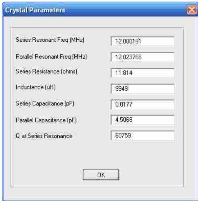
**Photo K:** 12 MHz crystal parameter measured data.
