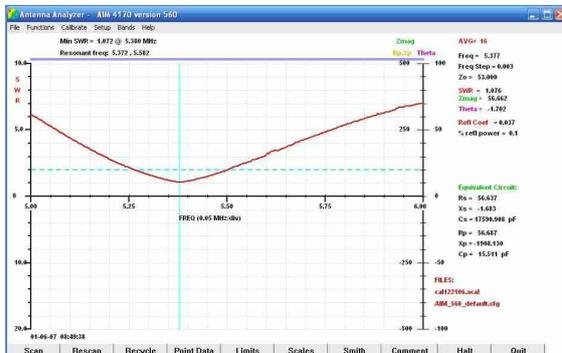
**Photo G:** 60-meter response of the Butternut vertical with 80-meter turns shorted.
