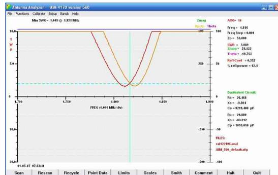
**Photo F:** Impact of shorting 80-meter turns on the 160 meter resonance region.
