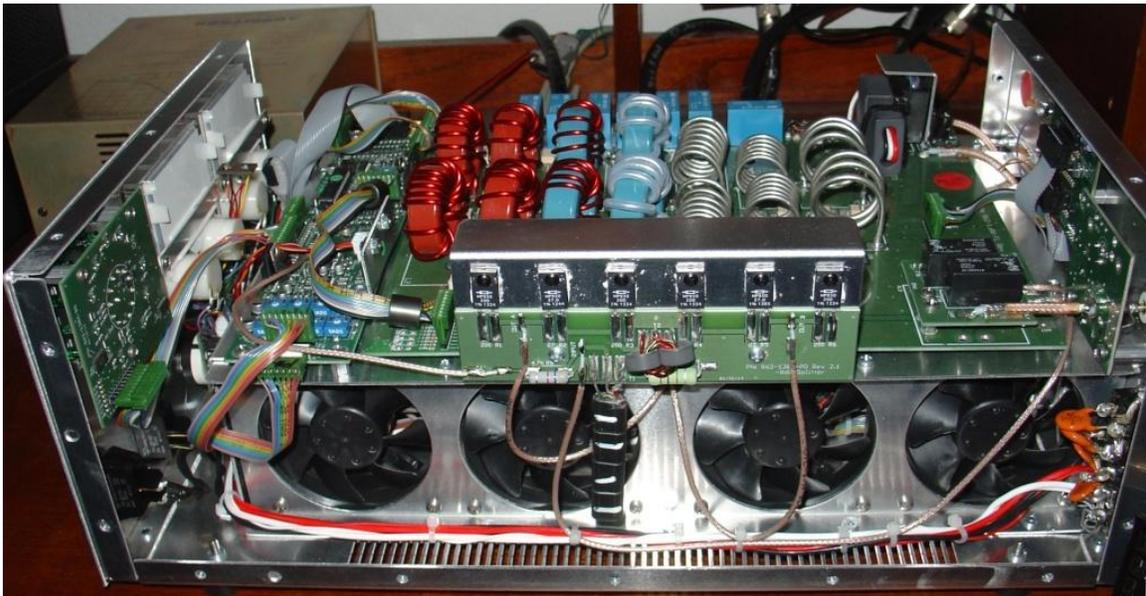
Figure 5: The ALS-1306 four 3" cooling fans.
