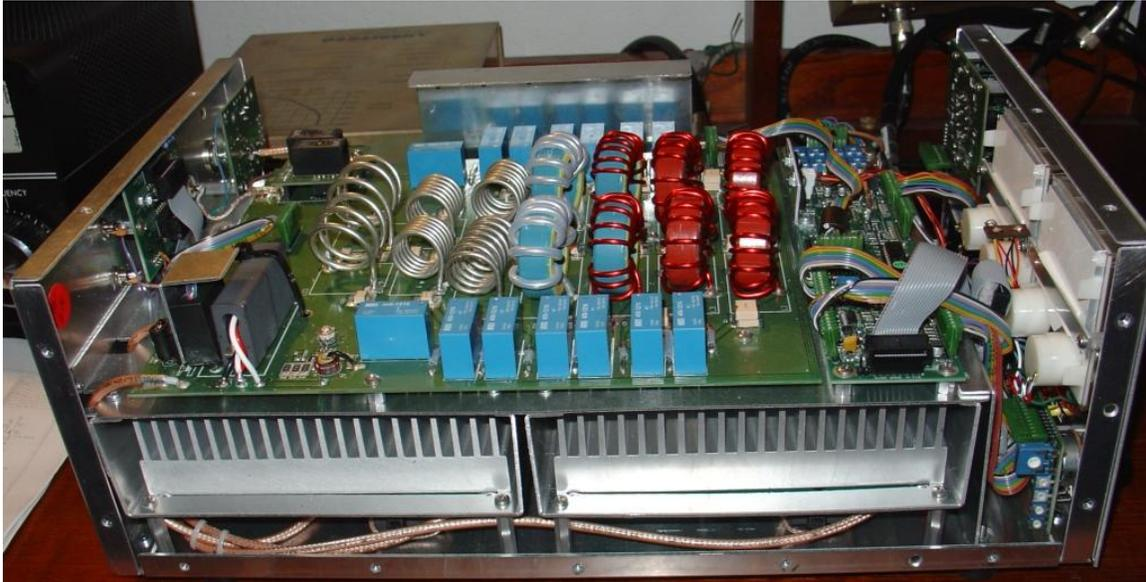
Figure 4: The two individual 600-watt amplifier heatsinks.
