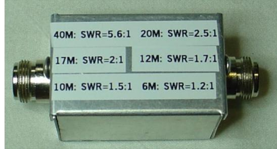
Figure 7: SWR degradation box - Internal      Figure 8: SWR degradation box - External
