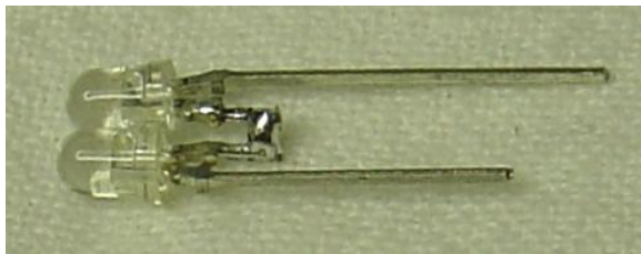
Photo B: 3mm LEDs soldered in series
