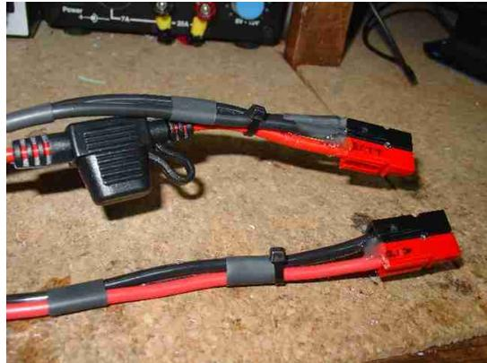
Photo D: Close-up of added Powerpoles
