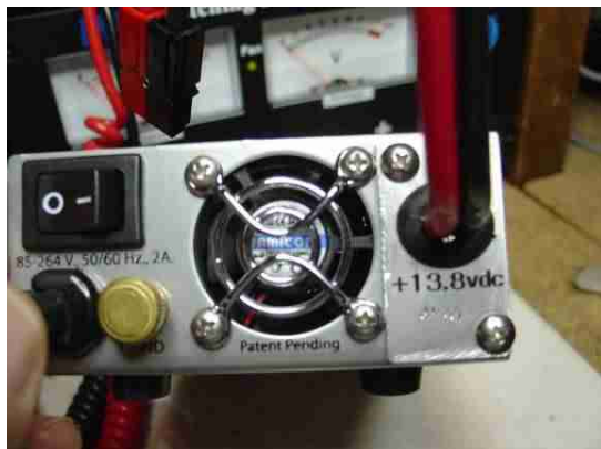
New rear plate and pendant cable
