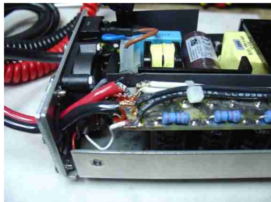
Pendant cable internal connection
