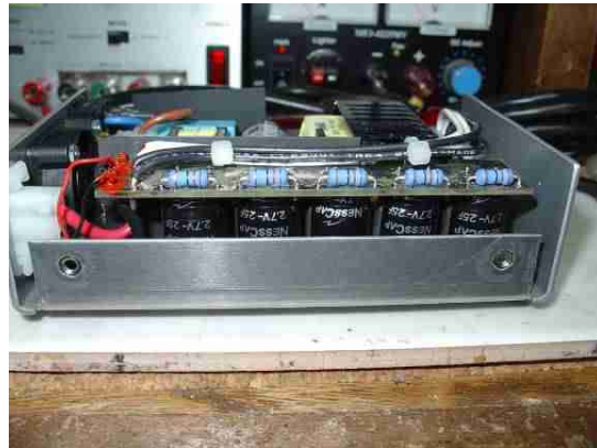
View showing the five 25-farad capacitors and equalizing resistors.
