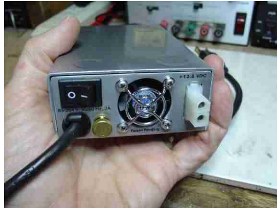
Backside showing the 20-amp Molex DC output connector. Gamma provides a matching plug (also available at Radio Shack).
