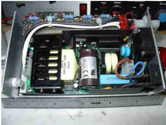
Inside view showing the 5-amp switching power supply in the front, and the capacitor bank assembly along the back.
