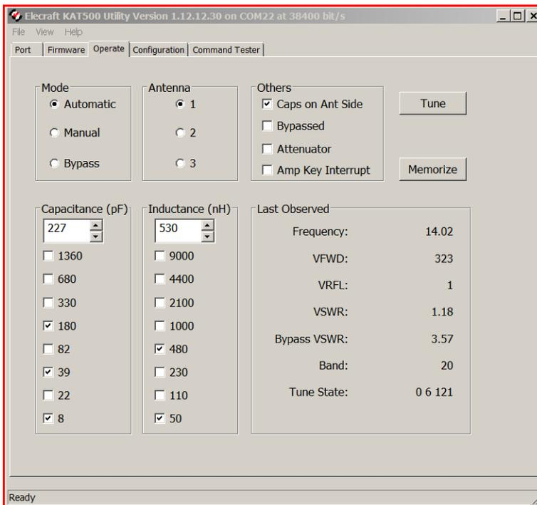
Figure 6: KAT500 tuning solution, 43-foot vertical on 20 meters
