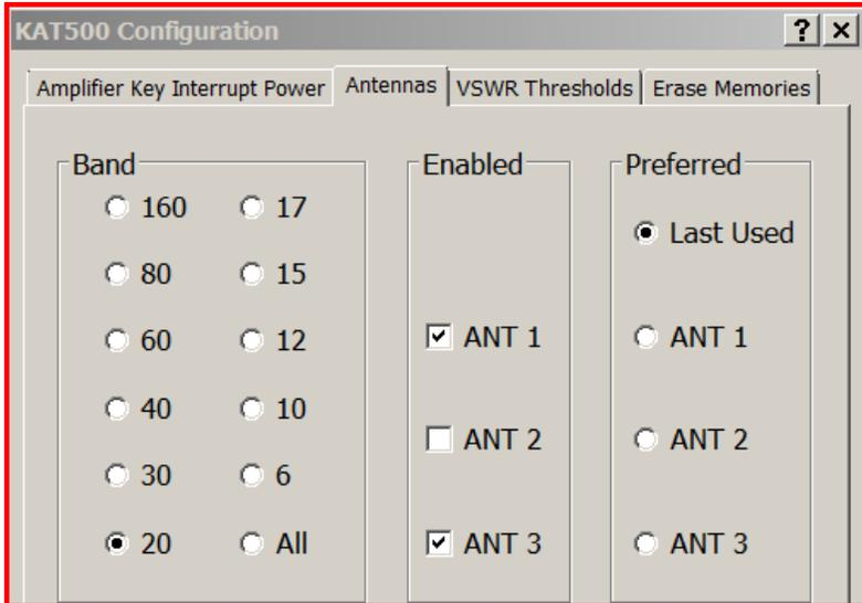
Figure 5: Antennas selected for 20 meters
