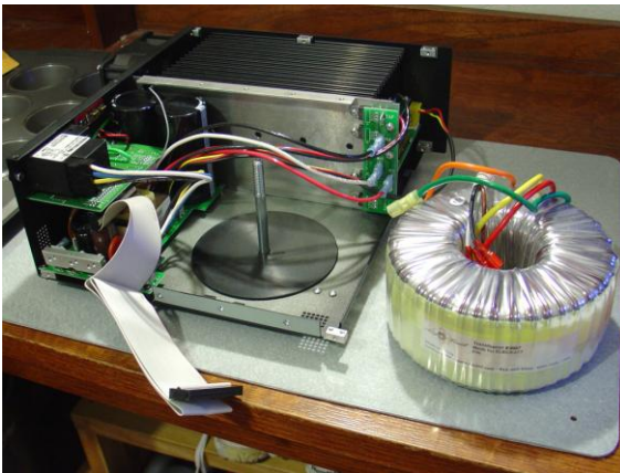
Figure 4: Ready for the power transformer. Left - I/O & Power Supply modules.
