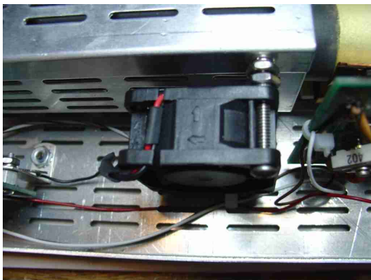
Photo A: Fan mounting details
