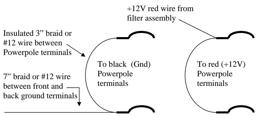
Figure 2 – Powerpole pin wiring
