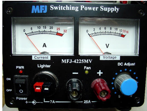
Powerpole plug assembly epoxied in place
