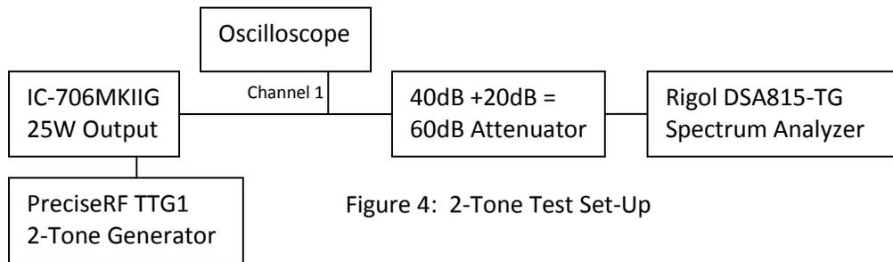
Figure 4: 2-Tone Test Set-Up
