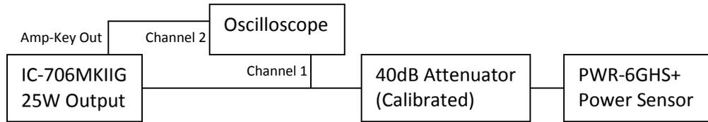
Figure 3: Amp Enable/Disable Test Set-Up
