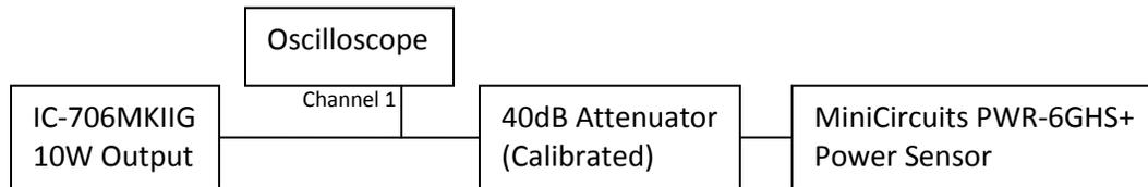
Figure 1: Frequency Response Test Set-Up
