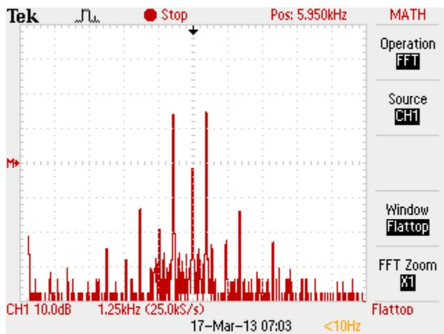
Figure 9: TBS1042 2-tone test FFT display
