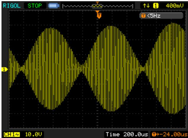
Figure 13: 2-tone RF-modulated transceiver output
