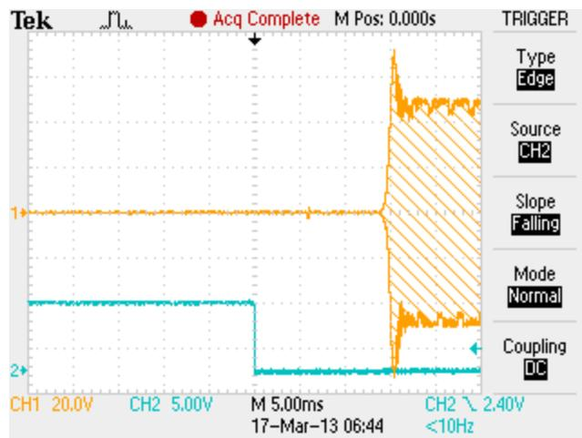
Figure 6: IC-706MKIIG Amp key-to-RF output timing
