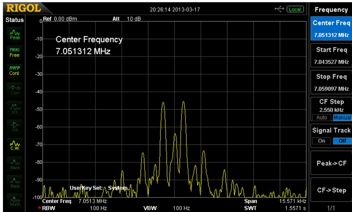
Figure 8: Spectrum analyzer display of IC-706MKIIG 2-tone test
