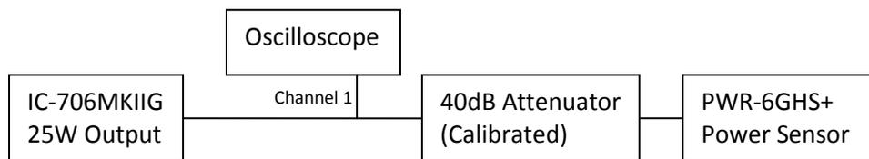
Figure 2: Transmitter Overshoot Test Set-Up
