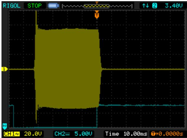
Figure 10: Amp enable-to-RF-to-amp disable timing. Again, note the first dit overshoot.
