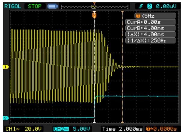
Figure 12: IC-706 amp disable/RF out timing
