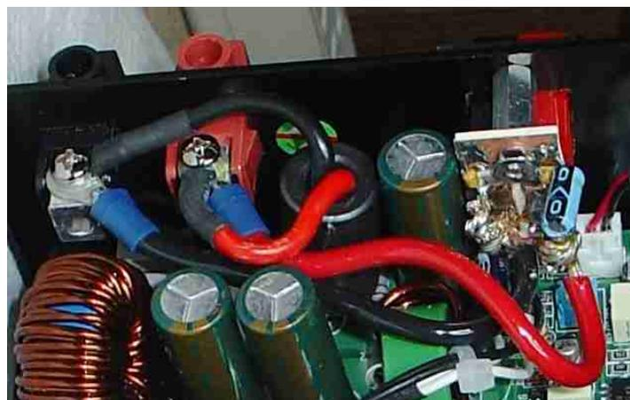
Photo J: Connector assembly mounted in place.
