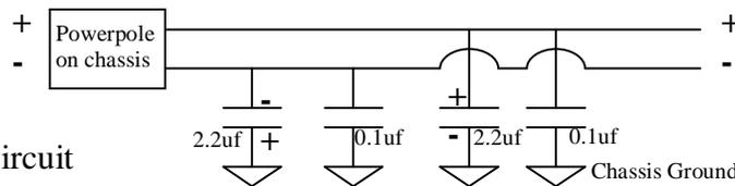
Figure 3: PCB Bypass Circuit
